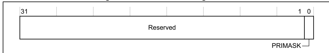
Figure 5. PRIMASK bit assignments
