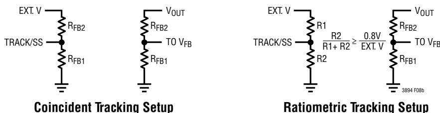
Figure 9(b): Setup for Ratiometric and Coincident Tracking
