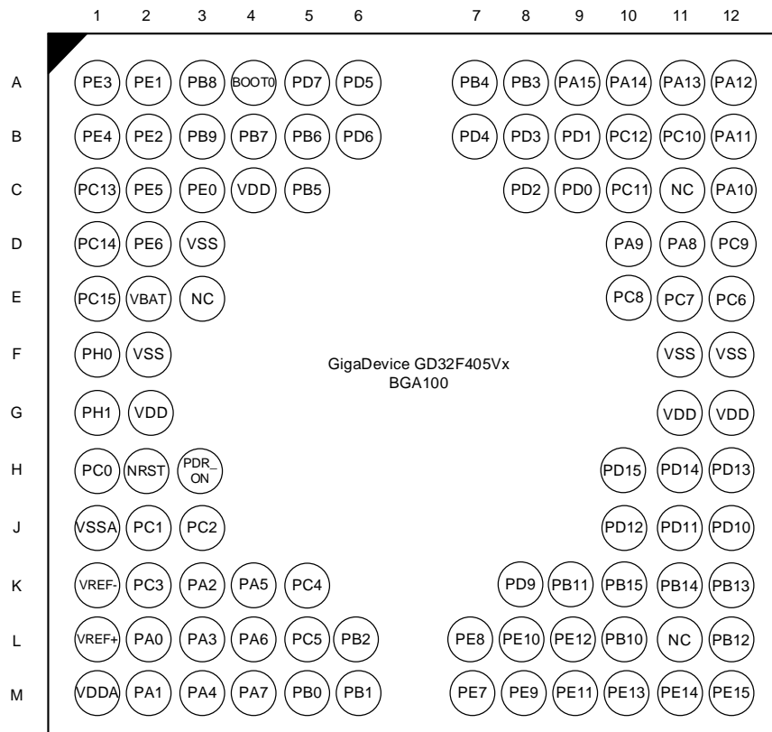
Figure 2. GD32F405Vx BGA100 pinouts
